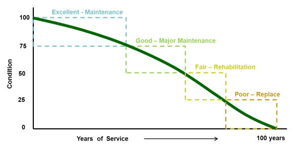
The following diagram depicts a general deterioration profile of a sewer main with a 100 year life.
