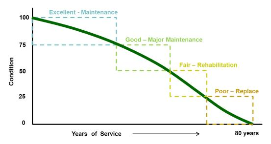
The following diagram depicts a general deterioration profile of a water main with an 80 year life.
